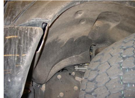
This is a picture of Lydall's wheel liner after 100% completion of vehicle level durability testing of a heavy-duty truck
