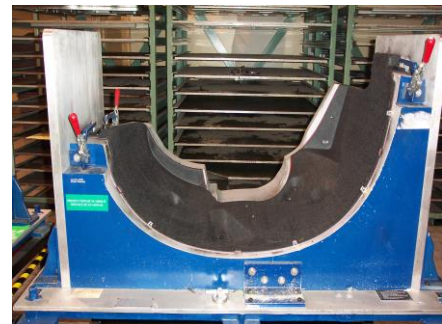
This is a picture of a production wheel well part placed in the check-fixture prior to packaging for shipment.
